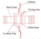
2. It had better put the outlet of the drain hose into the nearby drainage permanently, which can save the trouble that the drain hose has to be connected each time before use. If the drainage is far from the washing machine, it can be solved by connection of the drain hoses head with end to extend.
